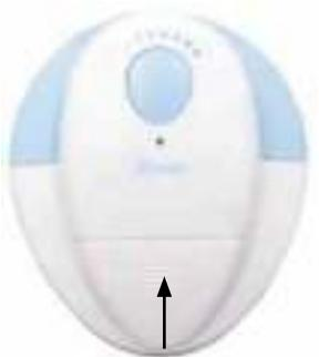
3. Slide the battery cover back onto the Baby Audio Amplifier.
