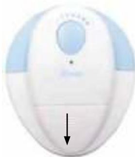
1. Slide the battery cover located in the front of the baby amplifier in a downward position.
