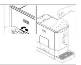
Place the appliance on a safe and stable surface with an easily reachable power supply and allow minimum distance from the sides of the machine.
