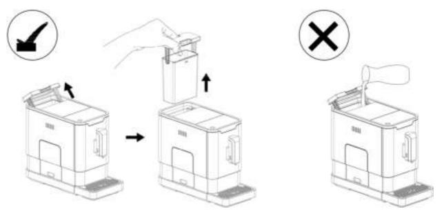
2. Rinse the water tank with fresh water and fill the tank to "MAX" level. Place it into the machine and make sure it is fully inserted.
