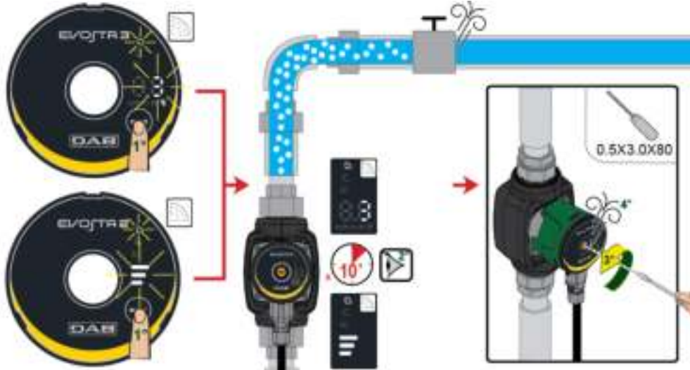
Figure 8: Venting of the pump
