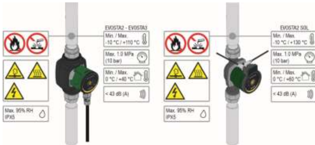
Figure 1: Pumped liquids, warnings and operating conditions
