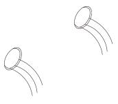
3. Wrap the S-connectors with teflon tape and then screw them into the pipes.
