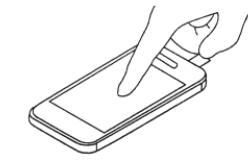
[EN] Lightly press the center of the Avanca® ToughGlass™ and wait for the adhesive silicone side to 'glue' itself to the screen. The oleophobic coating protects the glass from fingerprints.
