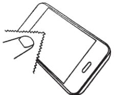
[EN] Use the alcohol swab to clean the screen of your device carefully. Use the dust removal sticker and the microfiber cleaning cloth for the finishing touch. Make sure that you do not touch the screen after cleaning.
