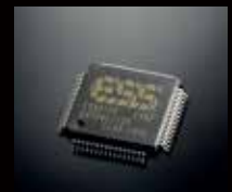
High performance ES9018 32-bit D/A converter
