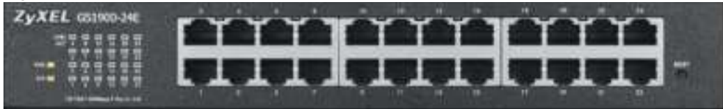
Figure 14 Front Panel: GS1900-24
