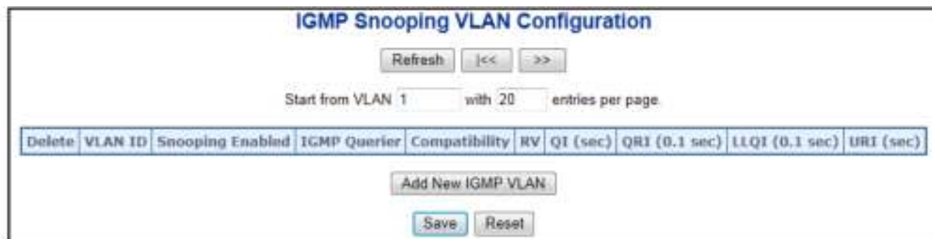
Figure 4-8-6: IGMP Snooping VLAN Configuration Page Screenshot
