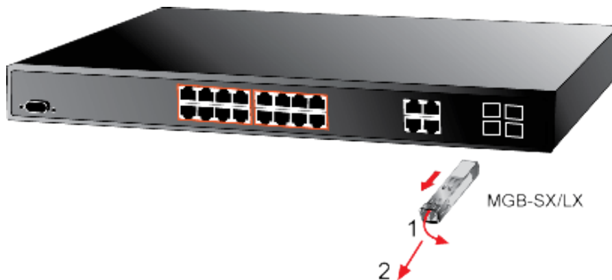
Figure 2-8: How to Pull Out the SFP Transceiver
