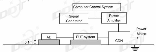
For analogue/digital data ports, if the cables may be longer than 3 m.
