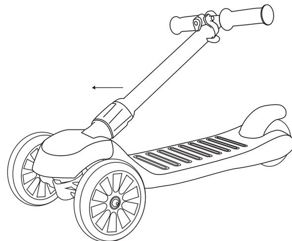
3. Fold the T-bar upwards
