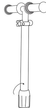
1. Unlock the T-bar by turning the knob clockwise.
