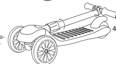
4. Turn the knob counterclockwise to lock the bar.
