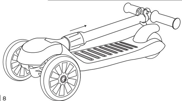
2. Pull the folding mechanism toward the T-bar until you can fold the bar upwards.
