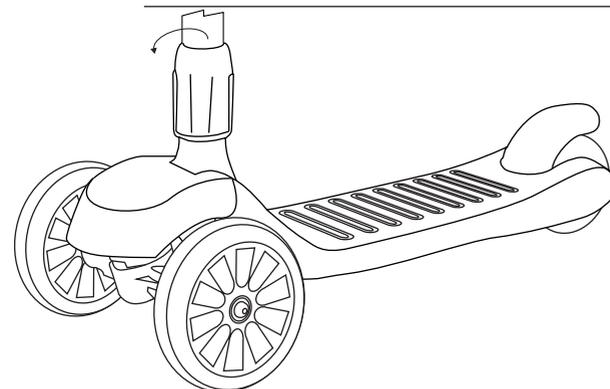
4. Turn the knob counterclockwise to lock the bar.
