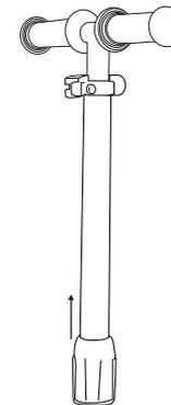
2. Pull the folding mechanism toward the T-bar until you can fold the bar downwards.
