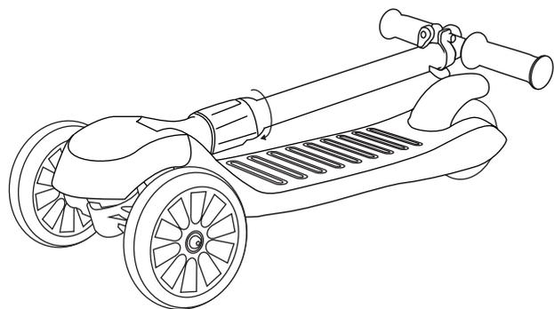
1. Unlock the T-bar by turning the knob clockwise.
