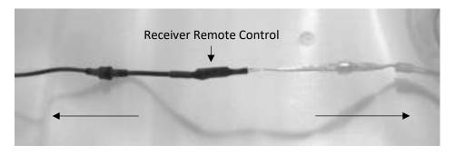
Left: black connection to power supply (2-pin plug) Right: transparent connection to the pool (4-pin plug)
