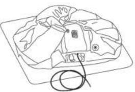
Open the air outlet on top of the filter heating element of the whirlpool and screw on the filling hose.
