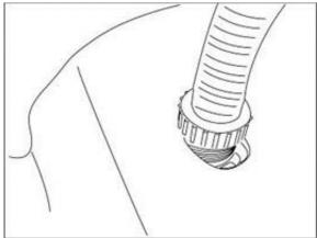
• Open the air valve on the whirlpool cover and attach the filling hose to the valve.
