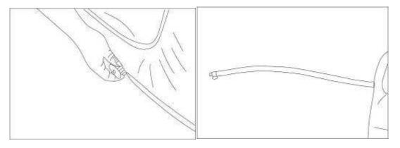
Then pull off the plastic plug on the inside. Now the water can flow out.
