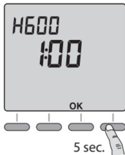
After installation you need to program initial settings. Turn the dial to the off position and press the right-hand button for 5 seconds until H600 code appears (maintenance menu reserved for the installer).
