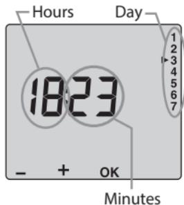
Turn the knob to ☉. The days flash. Press + or – to make your choice, OK to confirm it and go to the next setting. Repeat the operations to set the hours and minutes.
