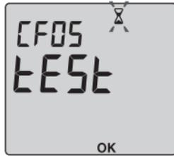
The transmitter sends a control signal to the receiver every 3 seconds. Check whether the receiver's light flashes on every reception.
