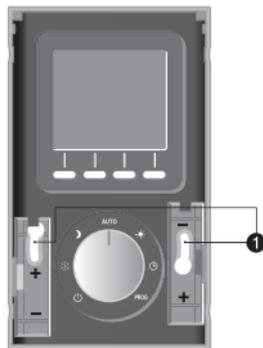
Wall mounting Secure the thermostat using the screws and pegs or fit onto a flush-mounted box (1, distance between centres 60 mm).
