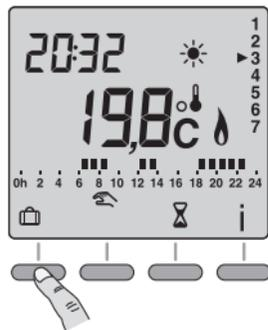
This mode is used to set a temperature (5 to 15°C) for a period that can be set from 1 to 365 days.
