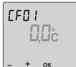
If there is a difference between the room temperature and the temperature indicated by the programmer, it is possible to correct it (from -4°C to +4°C in steps of 0.1°C).
