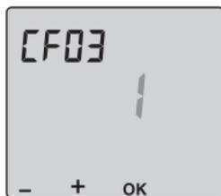
Early start means for the device to start heating in advance so that at the time set in the schedule you get the desired temperature, and not just start work (concerns the change from Eco to Comfort).
