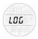
Smart Apnea can record the profiles of approximately 20 to 30 hours of diving, depending on the numbers of dives per session and the duration of each dive, assuming a sampling rate of 1 second. The information can be transferred using the optional USB clip to PC via the Dive Organizer software or to a Mac via the Divers' Diary software. In addition, Smart Apnea can show most of the information directly on the display.
