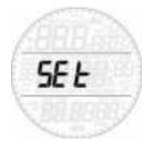
Smart Apnea's **SEt** menu allows you to change settings. Once inside this menu, press either button to scroll between two submenus: **SEt dIVE**, where you can set parameters pertaining to the dive, and **SEt tIME**, where you can set parameters pertaining to time and date.
