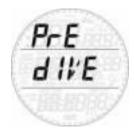
Press and hold the upper button to enter this menu and put Smart Apnea into the ready-to-dive mode.
