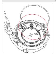
h) Position the cover onto the watch case and press it down evenly. Ensure that in the area of the screws the cover touches the watch case.
