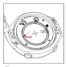
gl Position the new o-ring from the kit in the groove around the battery, ensuring that it sits towards the outer edge of the groove.
