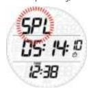
The stopwatch features also a split-time function: by pressing the lower button while the stopwatch is running, the time itself will freeze while **SPL** blinks in the top row and the stopwatch continues in the background. Every time you press the lower button the split time will refresh with the new value. Press and hold the lower button to exit the split-time mode. Note that while in split-time mode, the upper button has no function.
