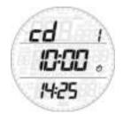
Press and hold the upper button and the minutes in the middle row will start to blink. Press the upper or lower button to modify the value, then press and hold the top button to confirm the value. Now the seconds start to blink.
