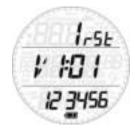
This submenu provides information about the hardware and software of your Smart Apnea and about the status of the battery (two segments inside the battery means the battery is ok, one segment means the battery is low but the watch functions as dive computer, one segment blinking means the battery is too low for use as dive computer).
