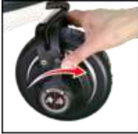
Figuur 51 Releasing the freewheel
