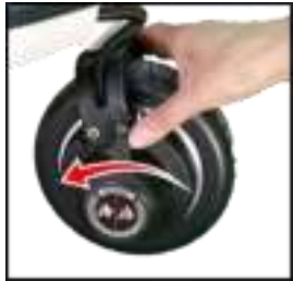
Figuur 52 Securing the freewheel
