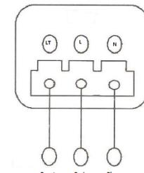
**Caution, never place 2 wires in 1 opening on the screw terminal.**
