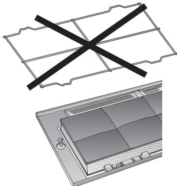
2. Place the activated carbon filter on the filter mat and clamp it in.
