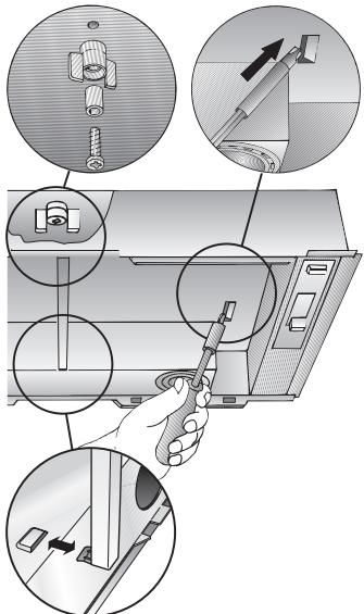
4. Tape over the activated carbon filter with the enclosed sealing strip.
