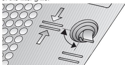
2. Press the retaining spring and remove the filter frame.
