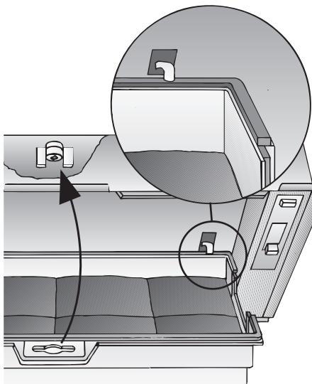
6. Re-insert the two filter cartridges.
