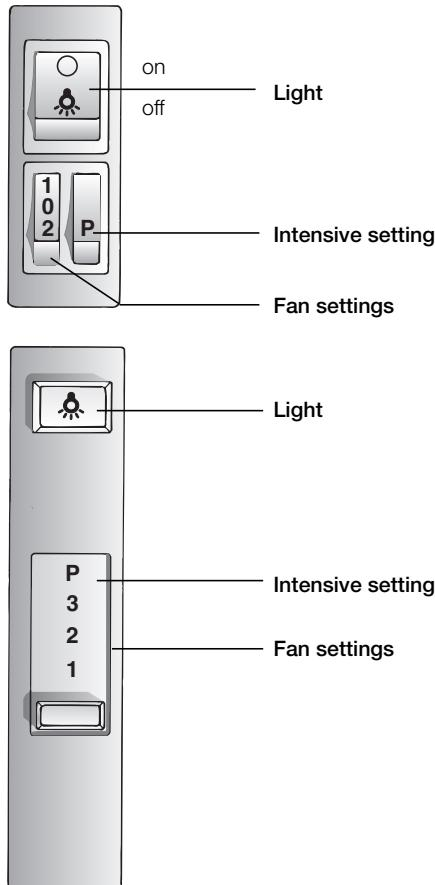
**Note:** The light can be switched on at any time, including when the vapour extractor tray has been pushed back into the hood.
