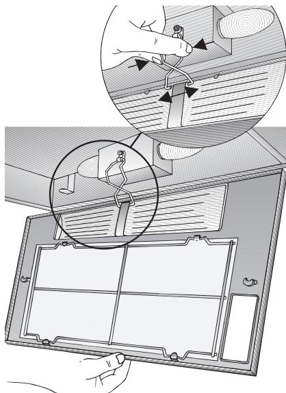
3. Remove the wire grille and replace the filter mat.
