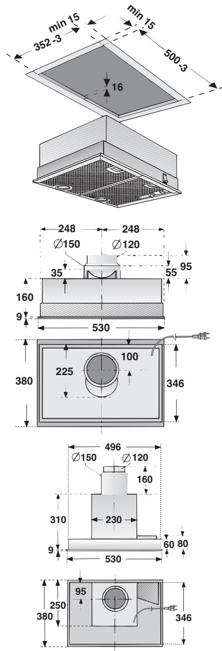
Extractor hood with slide control, 73 cm wide, 1 and 2-motor
