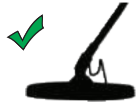
Correct search coil angle
