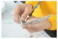
assemble flat-headed screws to the hanger with nuts in, but don't lock up yet
