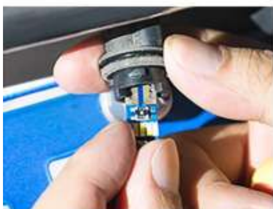
3. Insert directly the Audew T10 LED into the base(Non-Polarity)
