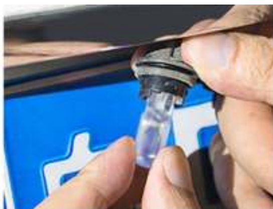
2. Remove the original halogen lamp from the base
