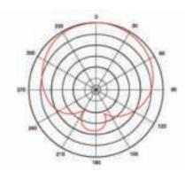
Directivity: Uni-directional Output connections: XLR (3-pin) Frequency Response: 50Hz - 15KHz
