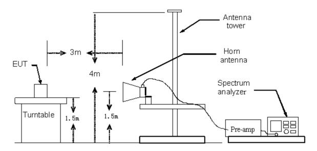
TEST PROCEDURE.1. Please refer to ETSI EN 300 220-1 (V.3.1.1) Sub-clause 5.2.2 for the measurement method.
