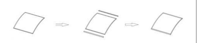
Insert aluminium bars on the two short sides.
