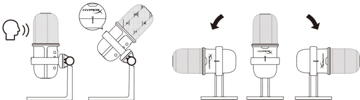
SoloCast should be placed with the front of the microphone facing the sound source. This is indicated by the alignment guide on both the microphone and the stand.
