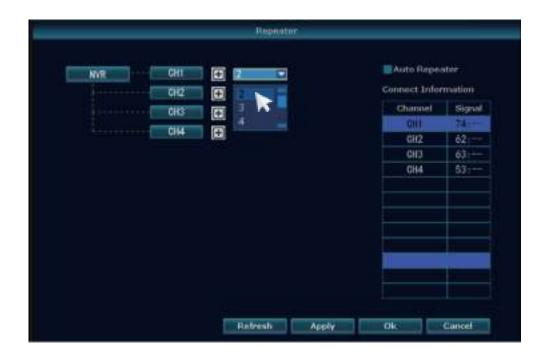
When you see your CH2 moves next to CH1, it means the extension is done. The CH1 will receive signal from the NVR recorder and send it to CH2! Well played!
