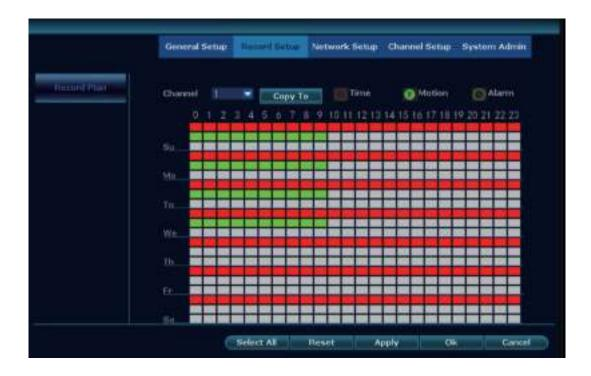
Alarm: When we set record period for "Alarm" and when the alarm is triggered, the NVR recorder will cut a piece of video (minimal video length: 30s) of the alarm and store the video separately.
