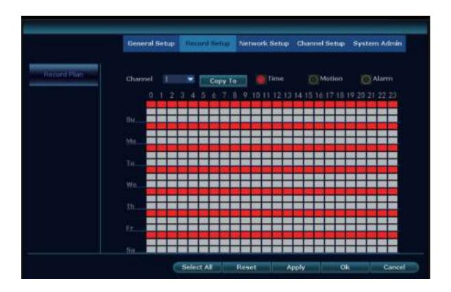
Motion: When we set a record period for "Motion" and when the camera detects a movement, the NVR recorder will cut a piece of video (minimal video length: 30s) starting at the moment of the detection and store the segment separately.
