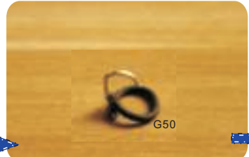
12. refer to get rid of the black rubber of the tail of G50 and then bend the tail
