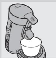
*Note: Always put a used coffee pod in the pod holder when you descale the machine. This pod serves as a 'filter' to prevent the sieve or hole in the pod holder from getting clogged with scale residue.*
