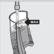
**2 Fill the water reservoir with cold water up to the MAX indication and put it back onto the machine.**
