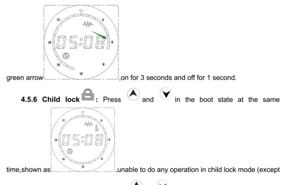
open and close), under child lock, press  $\checkmark$  and  $\checkmark$  3s at the same time can open the lock.
