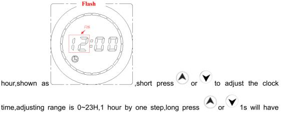
acceleration function.(No operation within 30s will exit time setting and enter minute setting).
