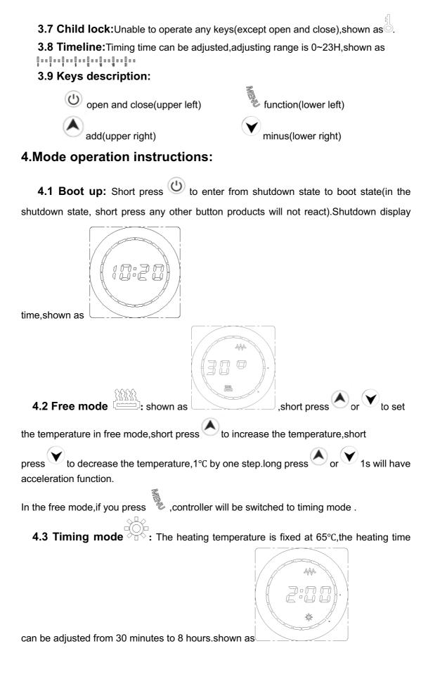
Short press or to set timing mode time, short press to increase time, short press to decrease time, 30 minutes by one step. Long press or 1s will have acceleration function. After the timer expires, the device will enter standby mode.
