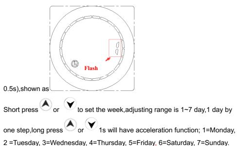
After setting up the week, short press to enter weekly program Setting (No operation within 30s will exit week setting and enters weekly program setting)
