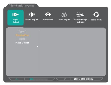
**3.** Press the **1** or **2** key to select the desired input source. Then press the **3** key to confirm the selection.
