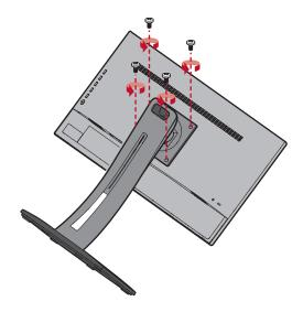
**4.** Pull down slightly to disengage the hooks and remove the stand.
