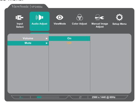
**4.** Press the **1** or **2** key to adjust/select the setting. Then press the **3** key to confirm.
