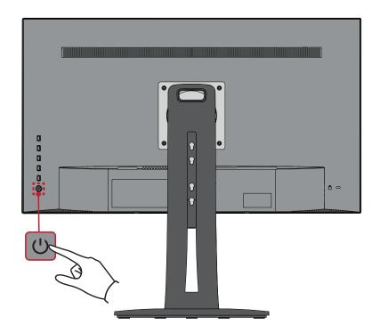
**NOTE:** The monitor will still consume some power as long as the power cord is connected to the power outlet. If the monitor is not being used for a long period of time, please disconnect the power plug from the power outlet.
