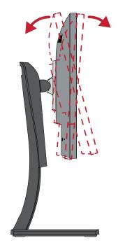
**NOTE:** When adjusting, support the stand firmly with one hand while tilting the monitor forwards or backwards with the other hand.
