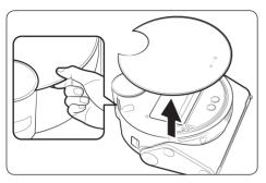
1 Detach the upper cover using the groove under the cover.
