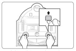
1 Push the Brush Cover Lock upward to unlock.
