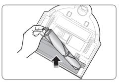
**3** Lift up the left side of the brush first and then pull the brush from the groove on the right.
