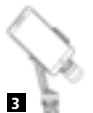
Fig. 3 If the smartphone tilts to the right, you need to move the phone a bit more to the left side up to the point where the gimbal can balance the smartphone. (Such as iPhone 5 / 5s and similar Android smartphones).
