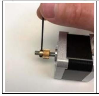
• Remove the extruder gear using the 1.5mm Allen wrench
