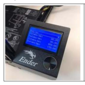
Extruder steps/mm needs to be calibrated. Good starting point is 130 steps/mm
