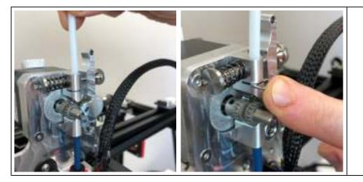
Insert the filament guide tube and secure it with the provided retaining clip
