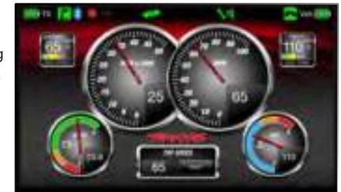
The customizable Traxxas Link dashboard delivers real-time rpm, speed, temperature, and voltage data.
