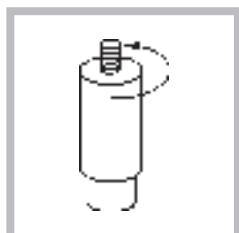
If it is necessary to level the appliance, screw the adjustable feet into the places provided on each corner of the base of the cooker (see figure).
