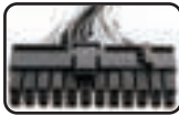
24P main power connector (Some models offer 4-pin module detachable design): For motherboard main power input and "I/O" control.
