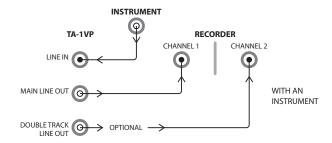
If you are recording directly to a tape deck or hard disk recorder, patch the output from an instrument into the TA-1VP's **LINE IN** and the TA-1VP's **MAIN LINE OUT** into your recorder. If you will be using the TA-1VP's Double Tracking function in stereo mode, patch the TA-1VP's **DOUBLE TRACK LINE OUT** to a separate channel on your recorder.
