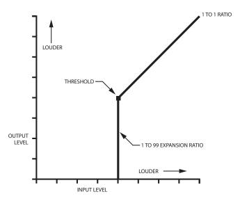
Sounds that are louder than the threshold get "through the gate" unchanged. Sounds that are below the threshold are not heard. Gates can be used to great effect in processing drum tracks where sounds from the other instruments in the drum set leak through the mike of the instrument being recorded. Gates are also used frequently to "gate off" a reverb tail or the ringing from an insufficiently damped drum head.
