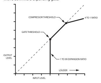
Using this setting, levels above the compressor threshold will be compressed at a 4 to 1 ratio. Levels below the compressor threshold but above the gate threshold will not be changed. Levels below the gate threshold will be gated out completely.
