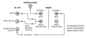
If (as is more common) your mixer has a single insert jack, you will need a "Y" cable with one 1/4" TRS (Tip, Ring,
