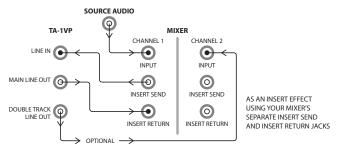
This is probably the most common setup for the TA-1VP. It will function as a pre-fader effect on one of your mixer's input channels.
