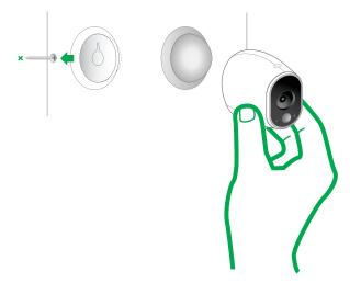
2. If you're mounting the camera to drywall, be sure to use the plastic drywall anchors that are provided.
