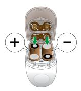
4. Insert two batteries near the compartment hinge. Pay careful attention to the orientation of the batteries when you insert them.
