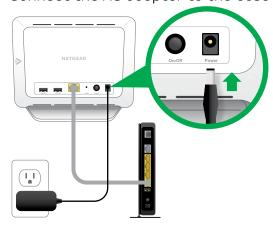
3. Plug the AC adapter into an electrical outlet.
