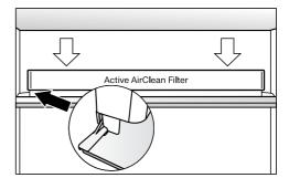
Place the holder in the middle of the protective strip at the back of the adjustable shelf so that it clicks into position.
