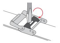
3. Insert the adjustment tool back into the slot and lock it down towards the strap.
