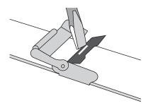
1. Open the top clasp. Insert the adjustment tool in the slot and lift it up.
