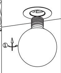
warning: when replacing a halogen lamp, wait for it to cool, for a minimum of 5 minutes
