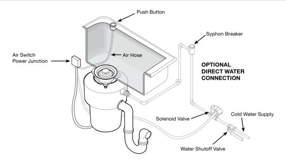
**PLEASE NOTE:** The Air Switch and socket need to be purchased seperately. For the wall mounting option a 20A ground connection is needed.
