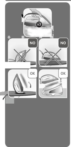
To release even more steam, press the steam trigger under the handle three times in quick succession for automatic sequential steam.
