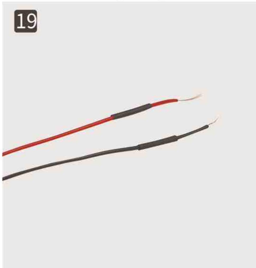
19 Cut off 2pcs shrinkable tubes(20mm) and cover the wire.
