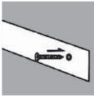
Screw the backing into the wall.
