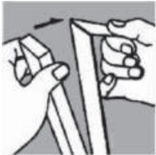
1. Pull the plastic separator out tightly and carefully, and separate the backing from the magnetic knife bar vertically to prevent injury.
