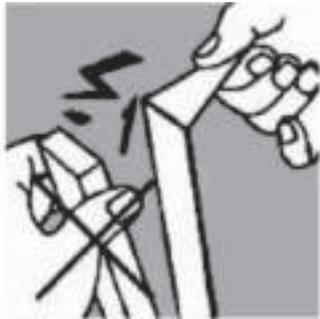
Be careful of the magnetic force from the magnetic knife bar to the backing, as it can cause injury to your finger or hand.
