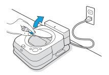
Add Braava jet® Hard Floor Cleaning Solution (if using).
