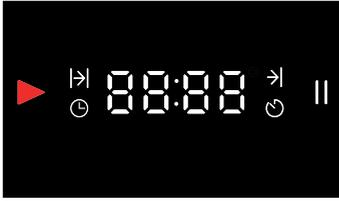
It is an electronic timer which makes the food to be cooked prepared at the time you desire. You should adjust the cooking duration of the meal and the time when you desire it to be prepared.
