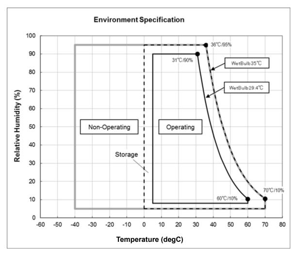
Figure 5 Limits of temperature and humidity
