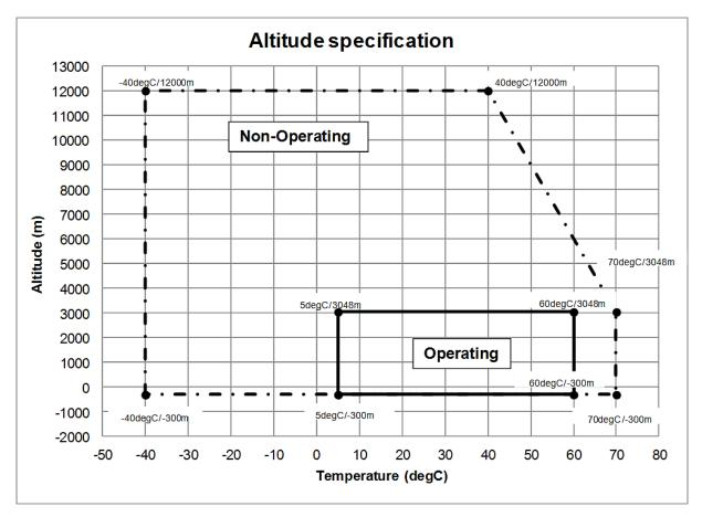
Figure 4 Limits of temperature and altitude
