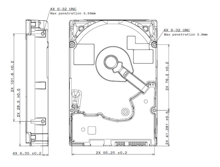
Figure 8 Bottom and side views with mounting hole locations (FIPS model)
