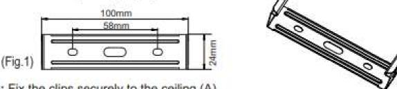
Step 3: Fix the clips securely to the ceiling (A)
