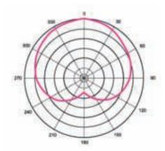
Directivity: Uni-directional Output connections: XLR (3-pin) Frequency Response: 50Hz - 13KHz
