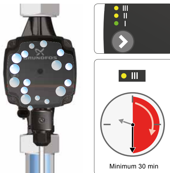
Fig. 7 Venting the pump
