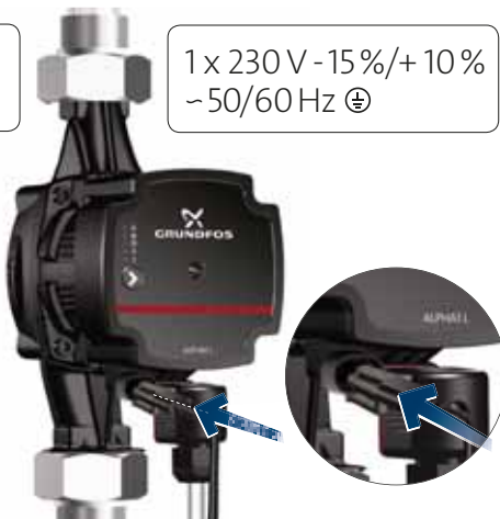
Fig. 22 Connecting the signal cable to ALPHA1 L
