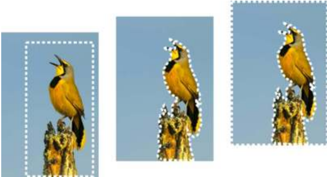
You can create a selection by using a Selection tool shape (left), by creating a freehand selection (center), or by using the Magic Wand tool to select specific areas of color or opacity (right).
